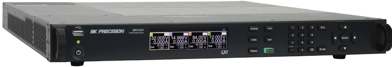
The MPS Series Modular System DC Power Supplies provide up to four output channels and 1200 W in a compact 1U form factor. Select from eight different modules with various voltage and current ratings to create a 1 to 4 channel DC power supply ideal for ATE system applications.
